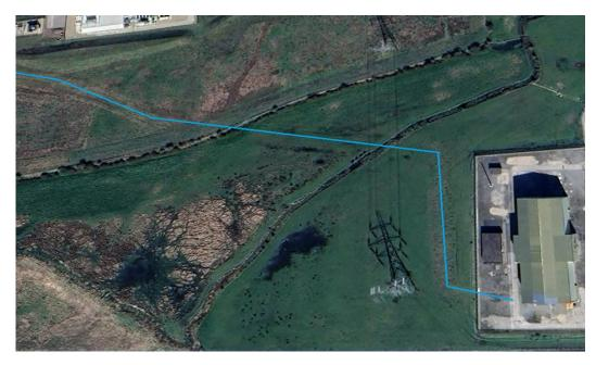
Figure 11 Route of power station buried cable
